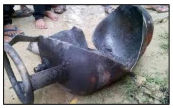
LPG cylinder explosions happen because of only internal pressure build-up and not due to any chemical reaction as external flame or air cannot enter a pressurized cylinder through the connecting tube or even through any leak therein to cause explosion.
